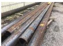
6 x LENGTHS BLACK STEEL PIPE<br>273.1OD x 12.7mm<br>3 @ 12m x 6.4mm<br>2 @ 12.7mm x 8m<br>1 @ 9.27mm x 9m |      |
