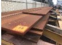
6 x LENGTHS STEEL PLATE<br>1 @ 530 x 25mm x 7.7m<br>5 @ 500 x 25mm x 8.5m                                 |      |
