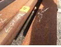
2 x LENGTHS RHS STEEL<br>1 @ 200 x 100 x 9 x 12m<br>1 @ 200 x 100 x 6 x 12m &<br>2 x LENGTHS SHS STEEL<br>1 @ 100 x 100 x 8 x 12m<br>1 @ 100 x 100 x 3 x 7m |      |
