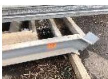
GALV STEEL STAIR SET<br>14 TREADS x 180 @ 3m (H) APPROX, 1130mm (W)                                                                                                                                                                    |      |
